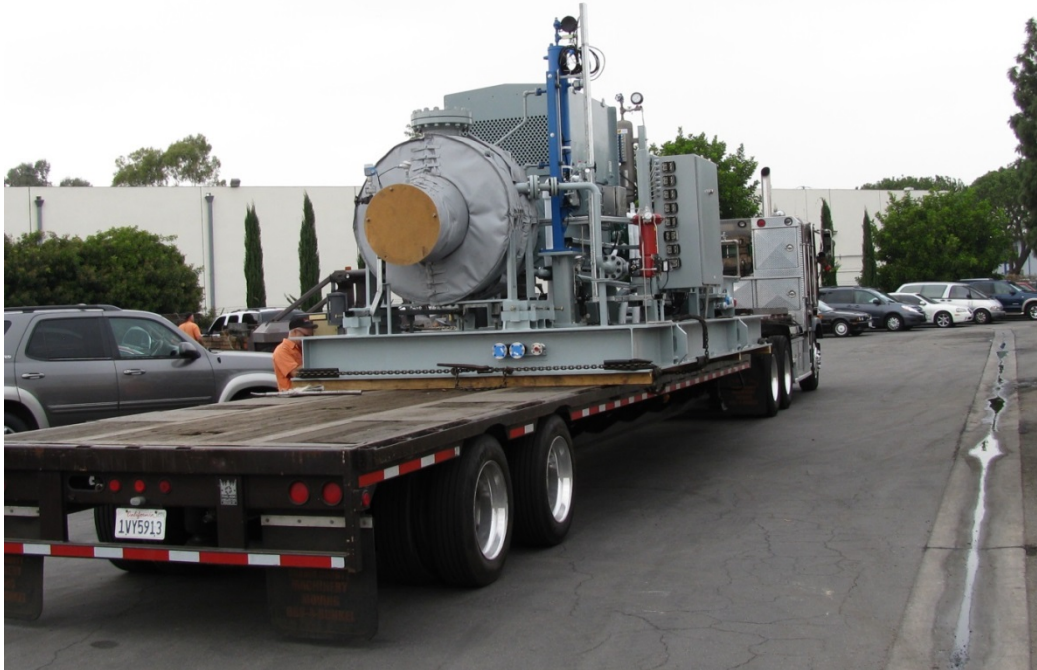
Figure 24 Variable Phase Turbine Assembly Loaded for Shipping
