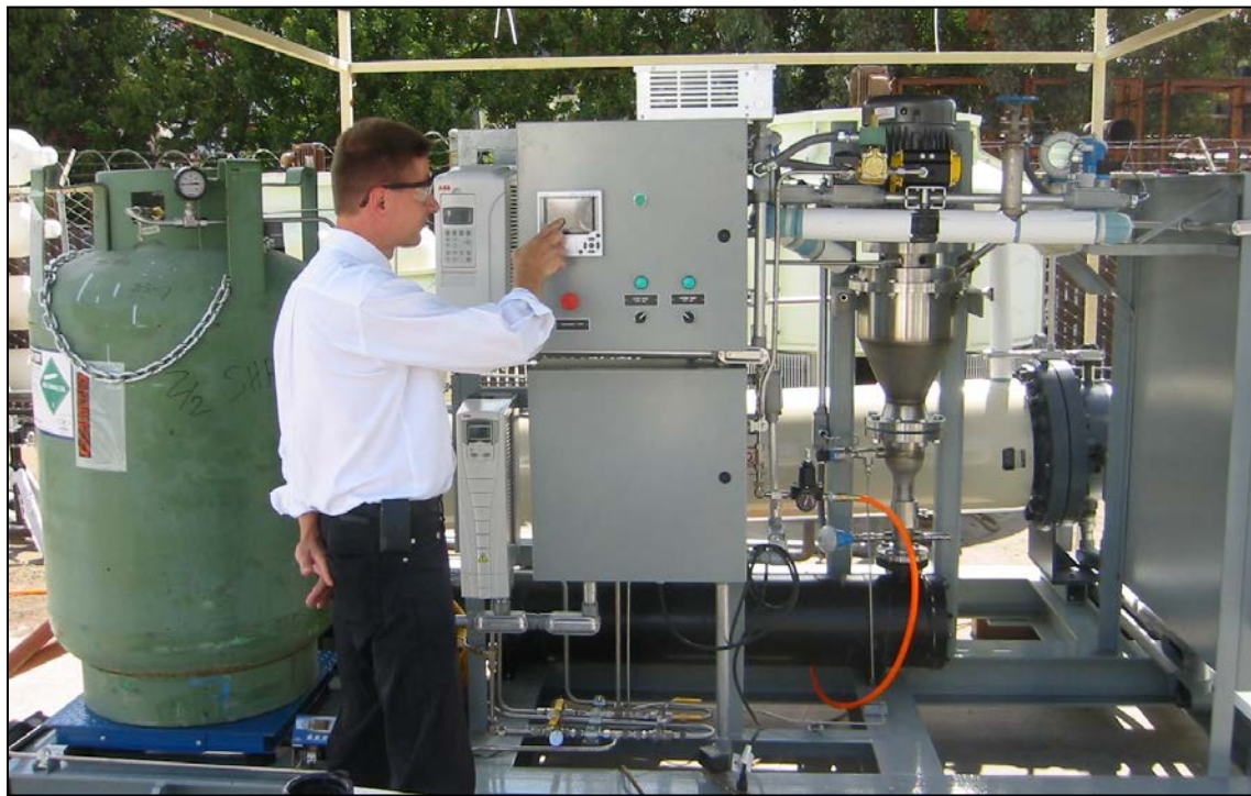
Figure 8 Variable Phase Cycle Pilot Plant Operating with R245fa
