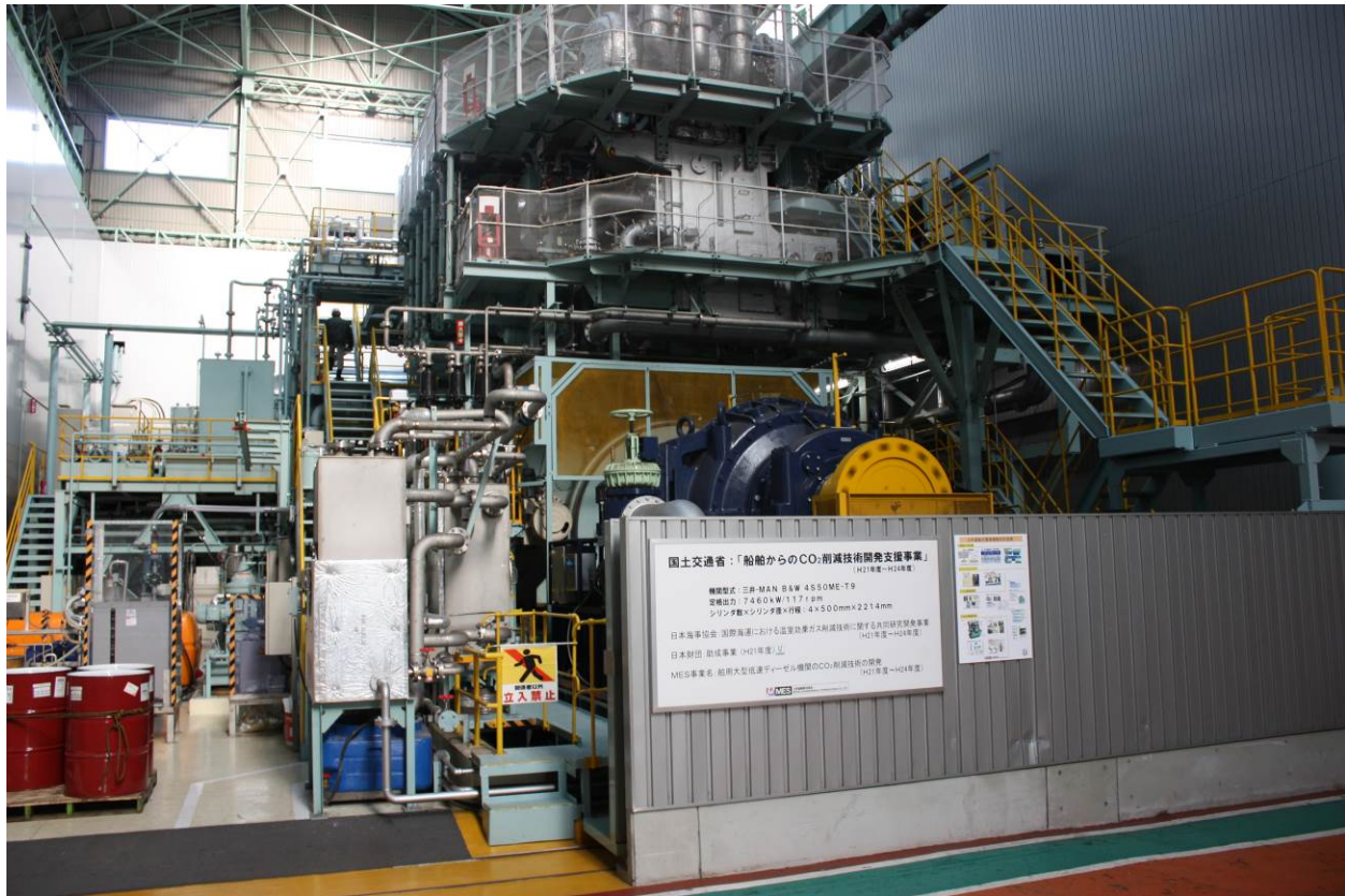
Figure 41 Ship Engine with Variable Phase Cycle Waste Heat Power System
