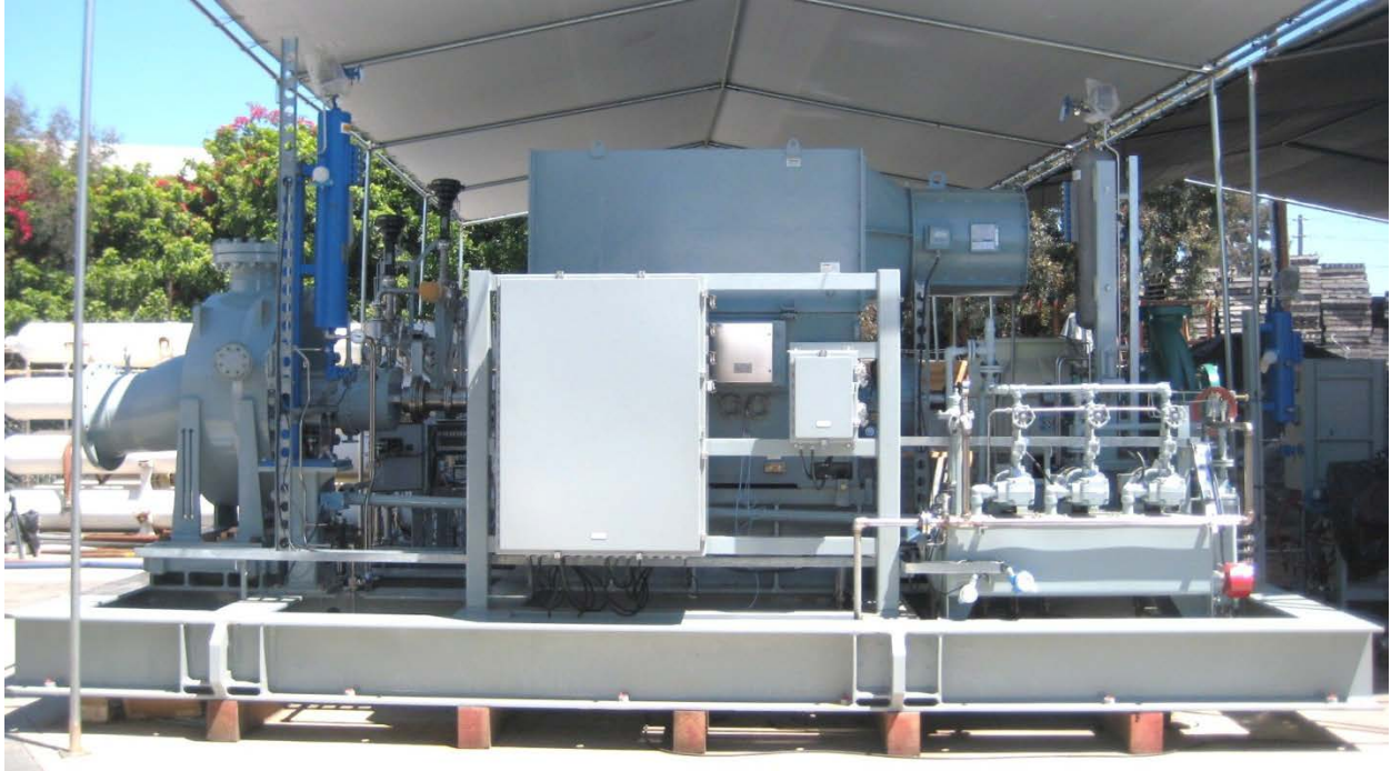
Figure 21 Rotating Assembly Mounted on Skid for Factory Testing
