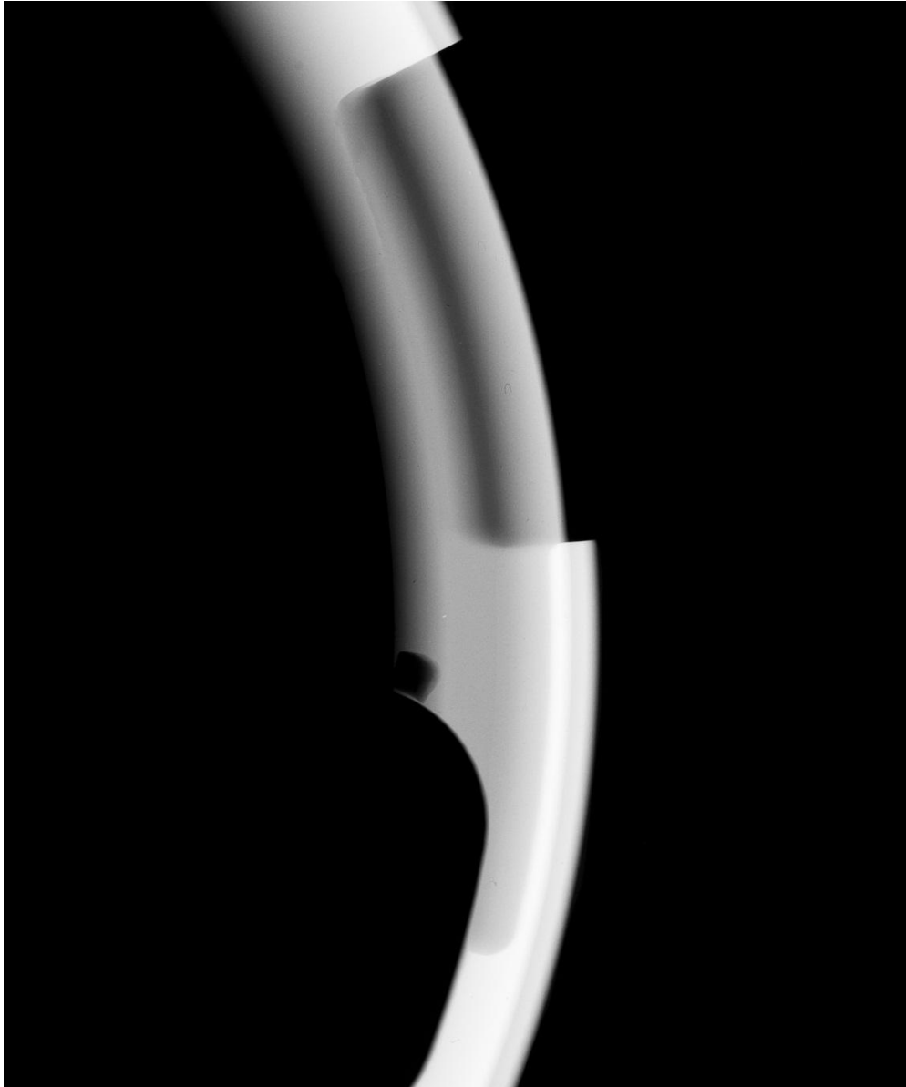
Figure 6. Close up of void present ring
