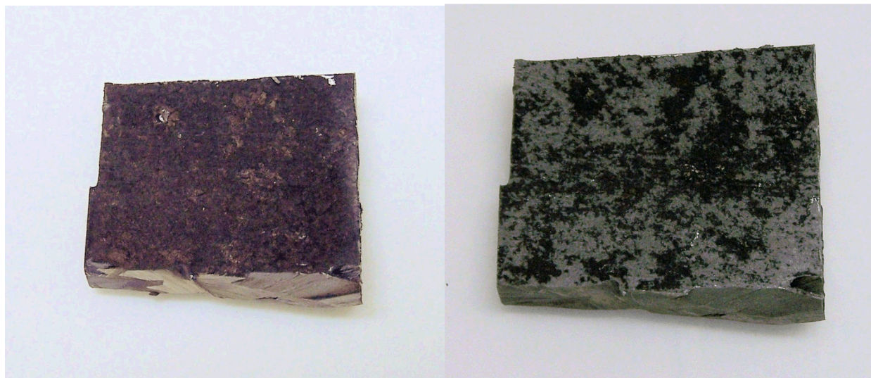
Figure 2-21. Photos of Coupon #2 from Jumper B – 2 Before (Left) and After (Right) the Ammonium Citrate Treatment Corrosion Removal Process.
