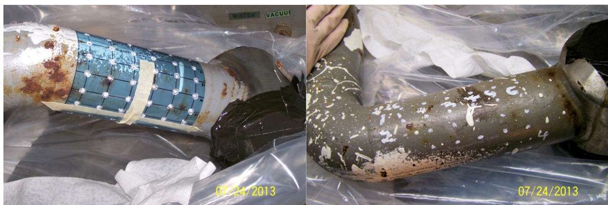
Figure 2-2. Photos of a Section of Jumper B – 2 During and After the Marking Process.
