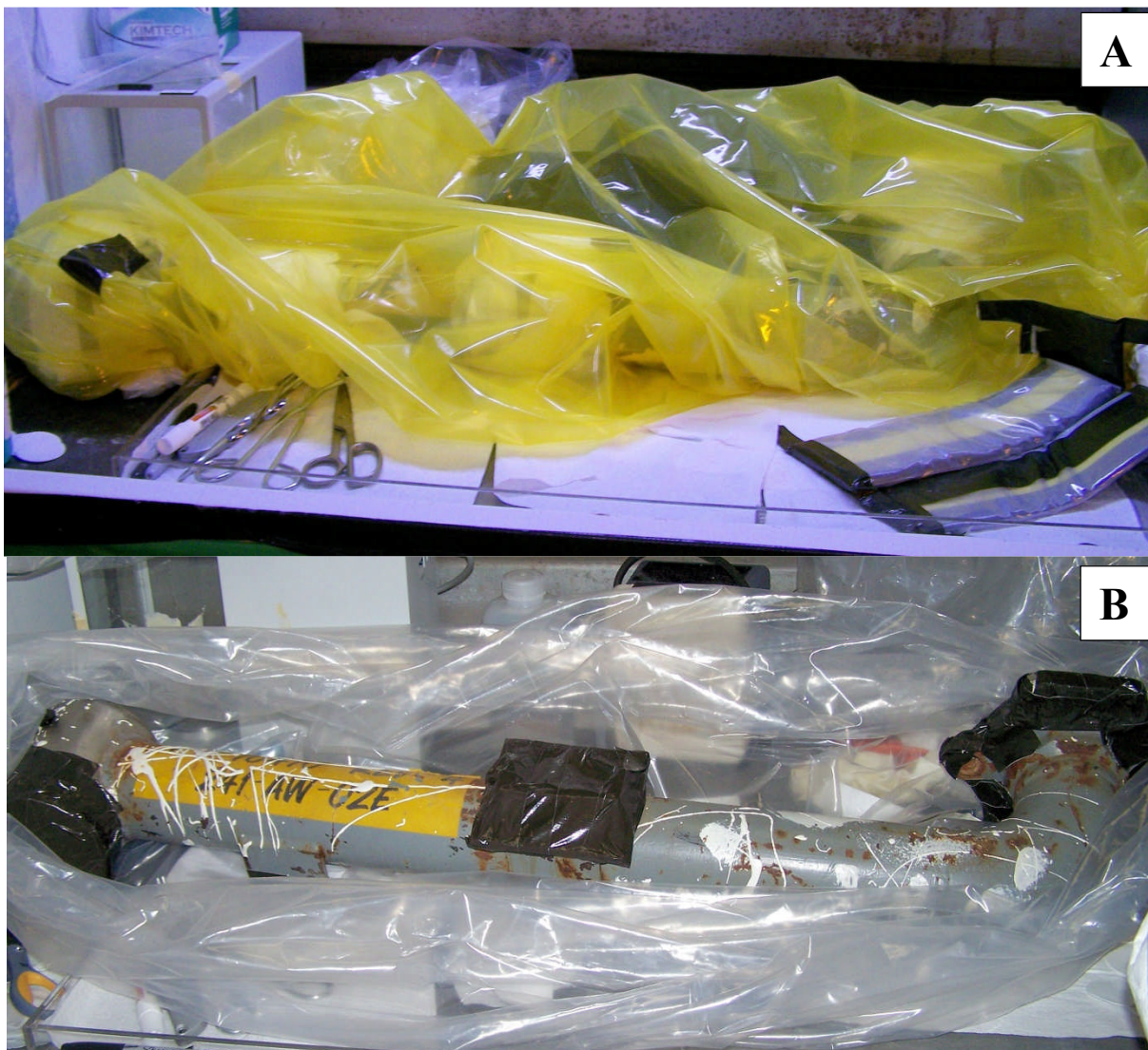
Figure 3-1. Photographs of the Larger Jumper 1 – 4 Section Before and After Removal of the Packaging.
