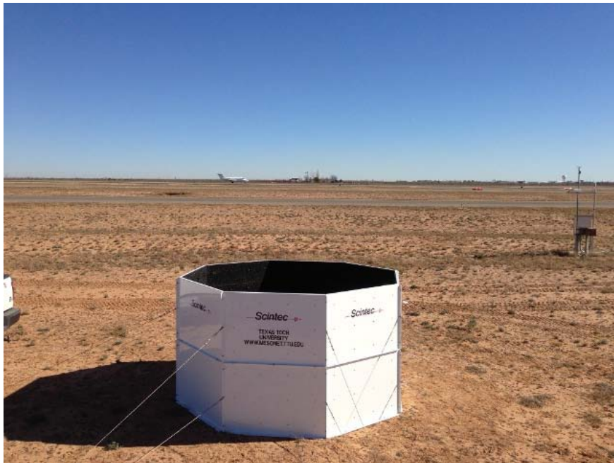
Figure 1.1.3.4. Photograph of the Midland SODAR (MSRT2) located on the main runway at Midland International Airport.
