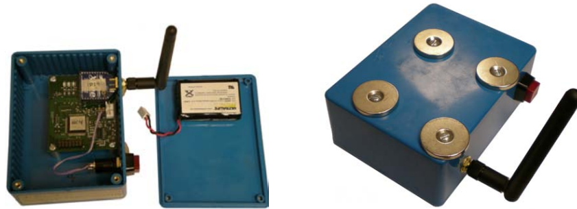
Figure 1.8.1.1. Sensor node circuit board with enclosure, lid contains a Li-Ion battery, and neodymium magnetic mounts.
