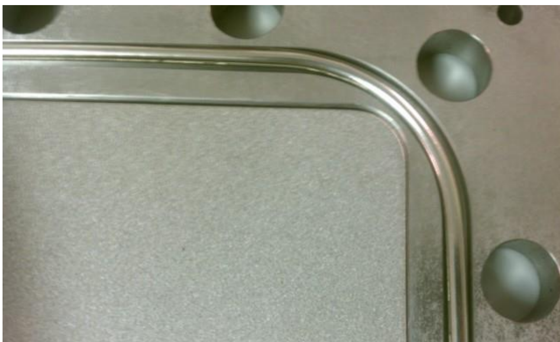
Figure 69. Module body with a spring energized seal.
