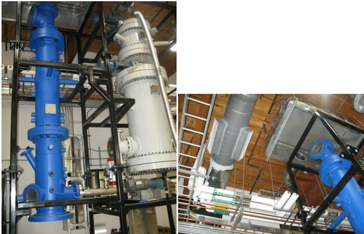
Figure 60. Auburn's gasifier (blue vessel) and a potential location for the membrane module.
