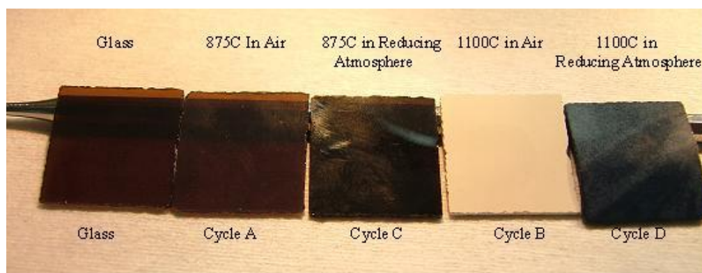
Figure 22. Picture of glass (annealed, at left) and ceramized CMAS-1/2 + Pd samples.
