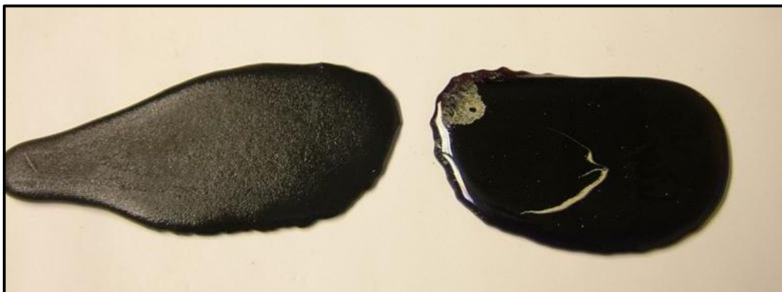
Figure 27. Photo of CMAS-21 and CMAS-22, respectively, from left to right. Slightly matte-like appearance of CMAS-21 likely due to retained small crystals in the as-cast glass.
