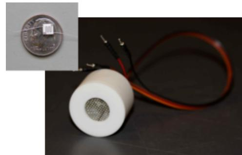
*Packaged Electrochemical H<sub>2</sub> Safety Sensor (above) and NREL rapid survey test, H<sub>2</sub> infiltration into fixed volume enclosure at 70% R.H. followed chamber purge (below).*
