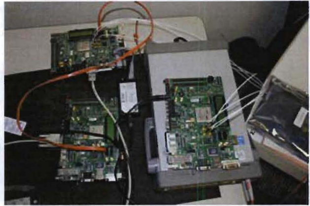
Figure 1. Photograph of the three node system currently in test. The red and white cables are the inter-FPGA network implemented with SATA and SMA cabling. In practice, these cards would be plugged into the PCI-E interfaces of the CPUs
