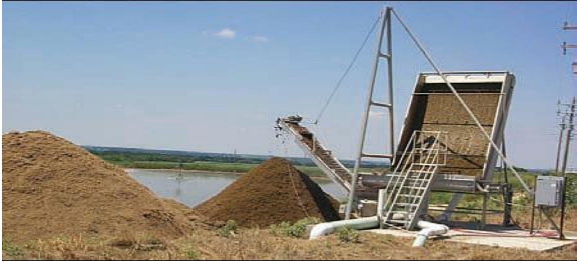
(Figure 2. Mechanical solid separation system. Water flows across a sloped screen that collects the solids. The solids then fall to the bottom and are collected by an auger and stacked using the flighted-conveyor separator.)
