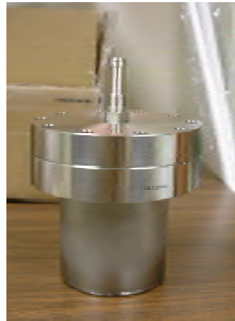
Fig. 6. Photographs of canisters built from high vacuum equipment to preserve noble gases that will degas from pore fluids in core samples.
