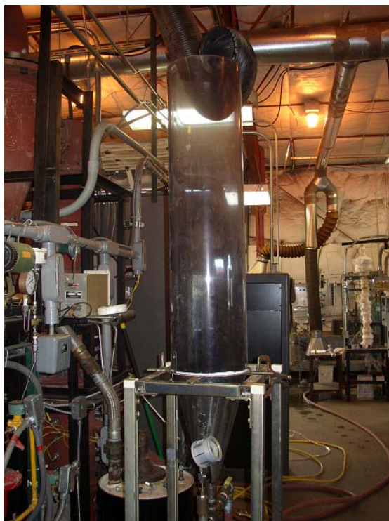
Figure 6. Second Cold Flow Model For Jet Spouted Bed Reactor
