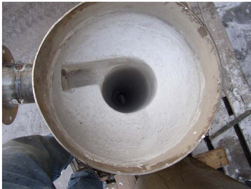
Figure 4. Internal view of cyclone cast in refractory.
