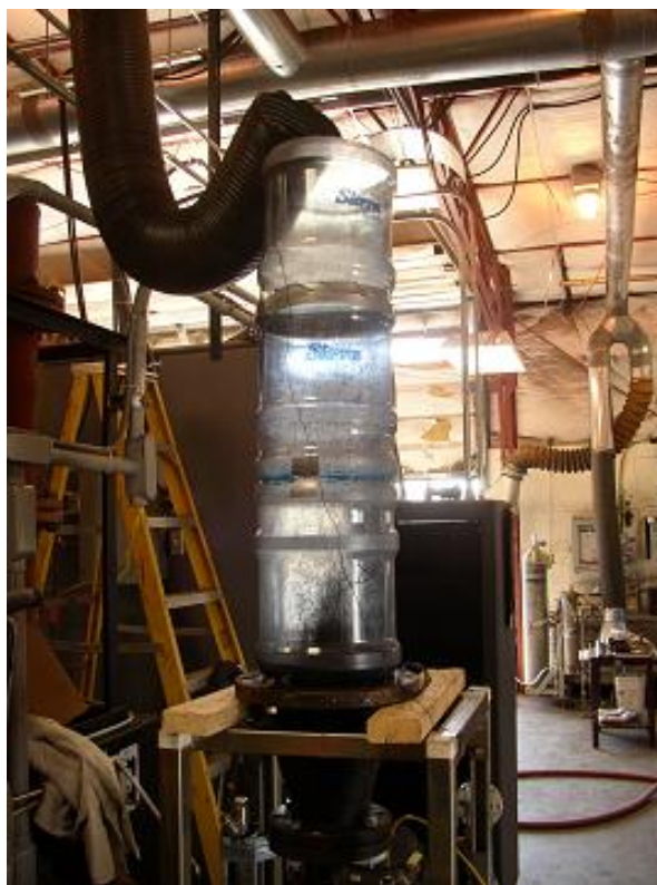
Figure 5. First Cold-Flow Model for Jet-Spouted Bed Reactor
