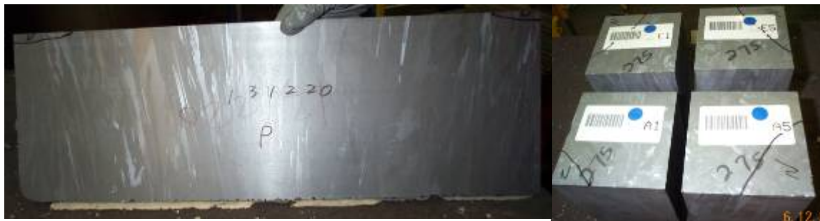
Figure 1.7: Side plates (left) and corner bricks (right) showing p/n transition at the very top of the ingot
