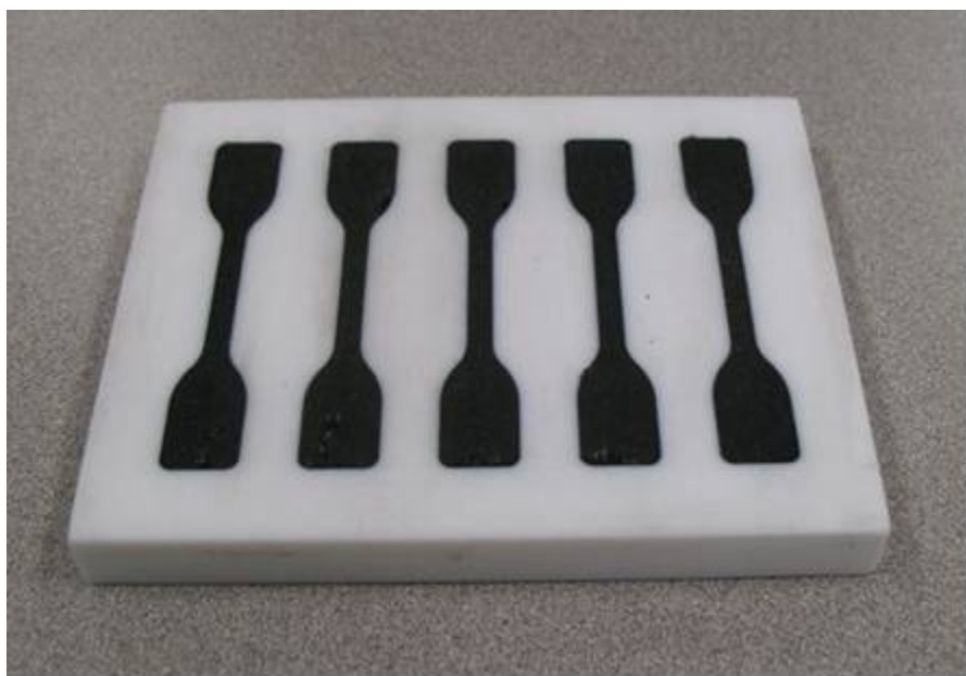
Figure 5.24: Example of sample preparation for frame adhesives: DIN 53504.
