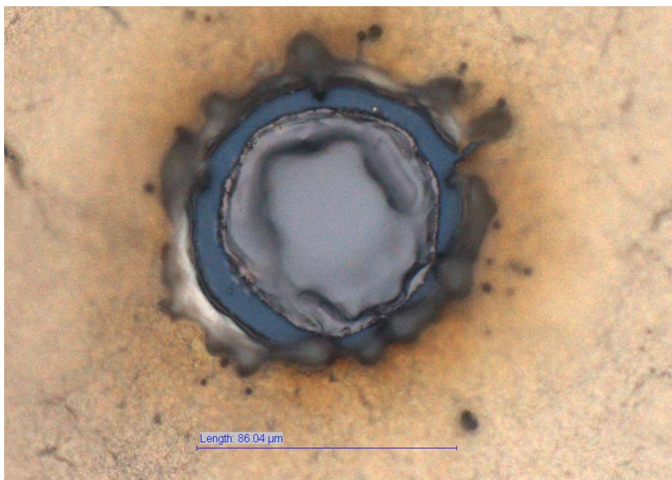
Figure 4.9: Photograph of a laser fired contact where the rim of the crater has been pushed across the blue dielectric ring (near the bottom right of the contact).
