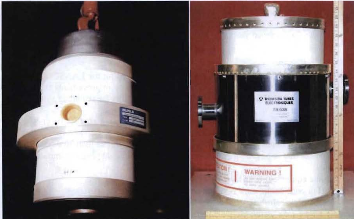
Fig. 2. The existing 201 MHz 7835 triode on the left and the new TH628 Diacrode® on the right.
