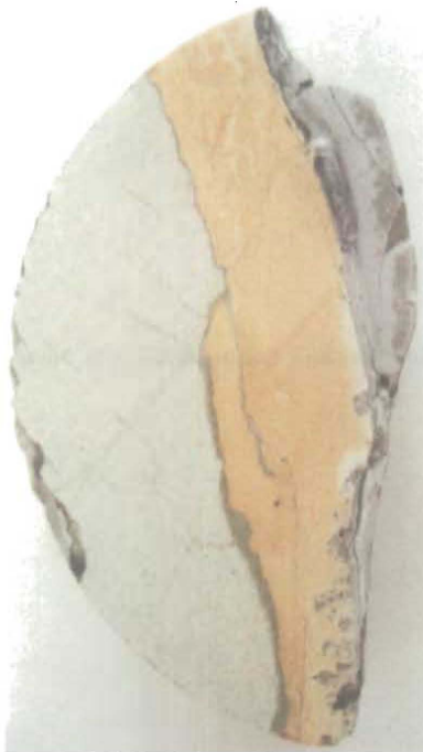
Figure 1. Polished face of cement recovered from a wellbore at the SACROC Unit in west Texas. Orange alteration reflects carbonation from fluids migrating along the cement-caprock interface on the right side of the image (about 5 cm in length). A narrow, dense, siliceous deposit separates the orange altered cement from relatively unaltered gray cement (from Carey et al. 2007).
