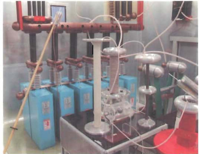
Fig. 5 LENS 24 \mu\text{F} , 100 kV self healing capacitor bank (~2 M width)
