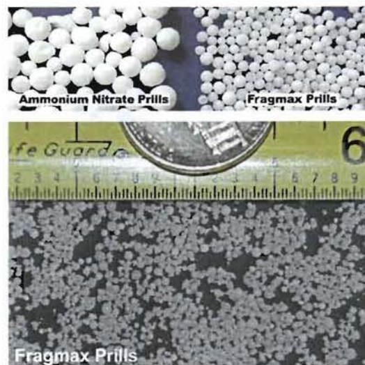
Fig. 8. Prill photos demonstrating size differences between standard explosive grade PPAN and Fragmax specialty prills. (Upper photo taken by manufacturer Dyno Nobel.)
