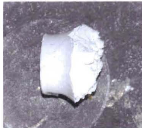
Fig. 3. Image of a recovered PBX-9501 acceptor pellet in the gap test with a no-go result.
