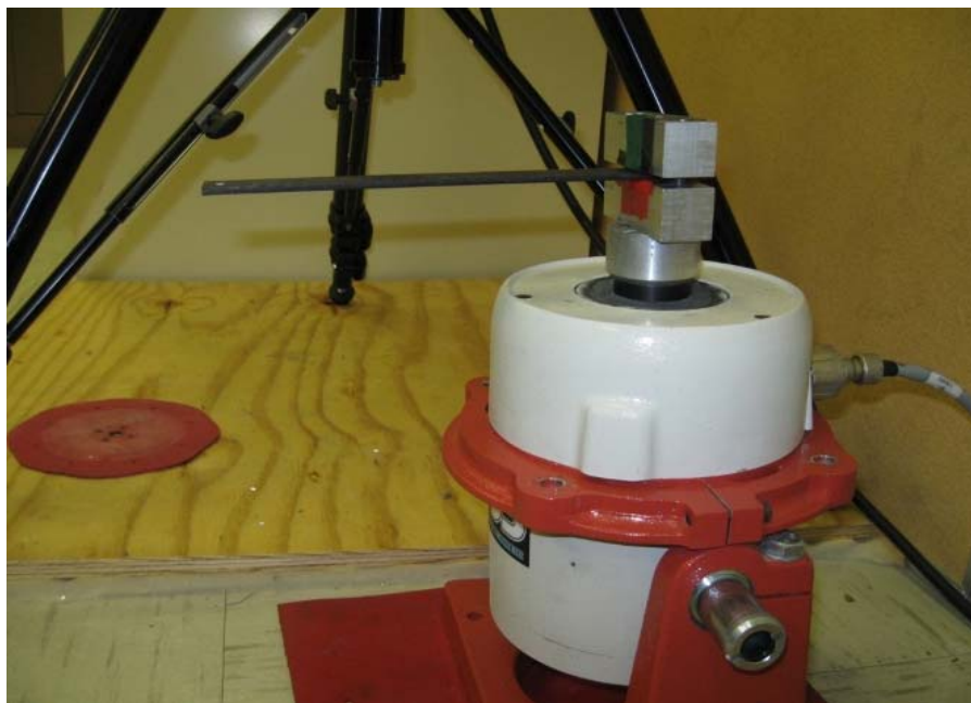
Figure AU-7: A test piece in between clamp, which is attached to moving platform of the shaker.
