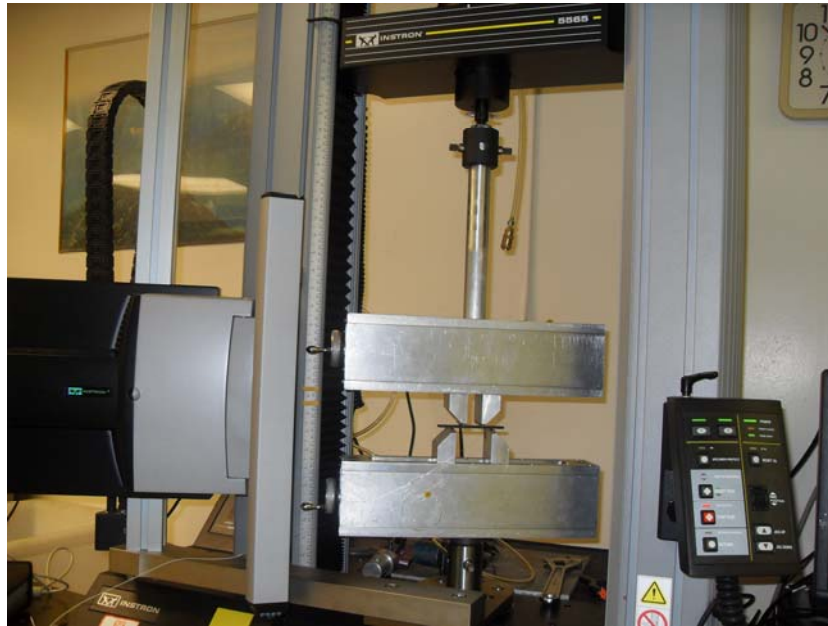
Figure AU-3: Four-point bending of a composite coupon.
