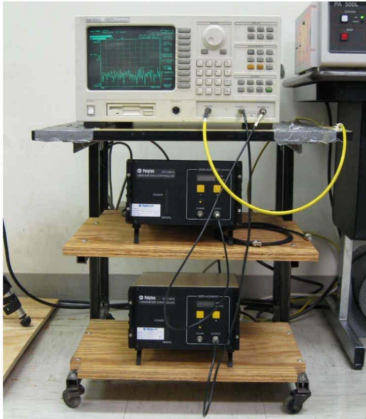
Figure AU-8: The analyzer connected to the vibrometer controllers and the yellow cable for the source signal.
