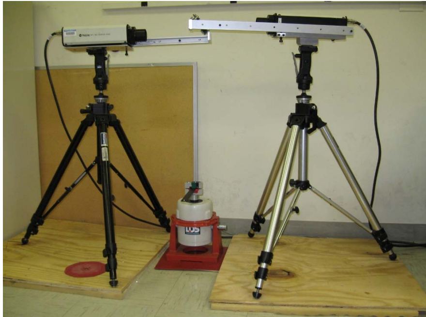
Figure AU-6: Two laser sensor heads with the shaker in between.
