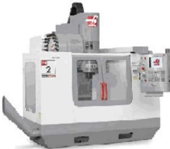
Figure MR1.1. Computer numerical control (CNC) drilling machine with 3-axis control (Photograph from Haas Automation, Inc. California, USA)
