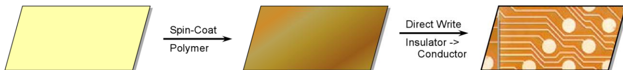
Figure 1. Schematic depiction of direct writing. Conversion of an insulating material directly into a conducting material upon application of light would require no metallization, strip or lift-off steps.
