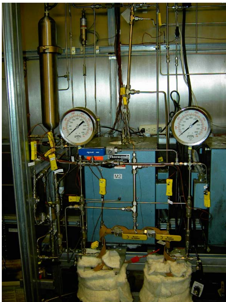
Figure 2. Micro-scale Hydrothermal Liquefaction System
