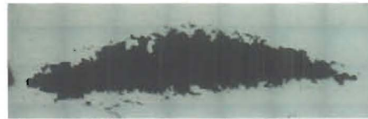
Figure 6. RD-0 target metallography of damage surface area.
