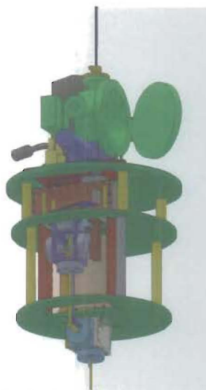
FIGURE 7. Proposed design for cryostat with load lock for rapid sample exchange
