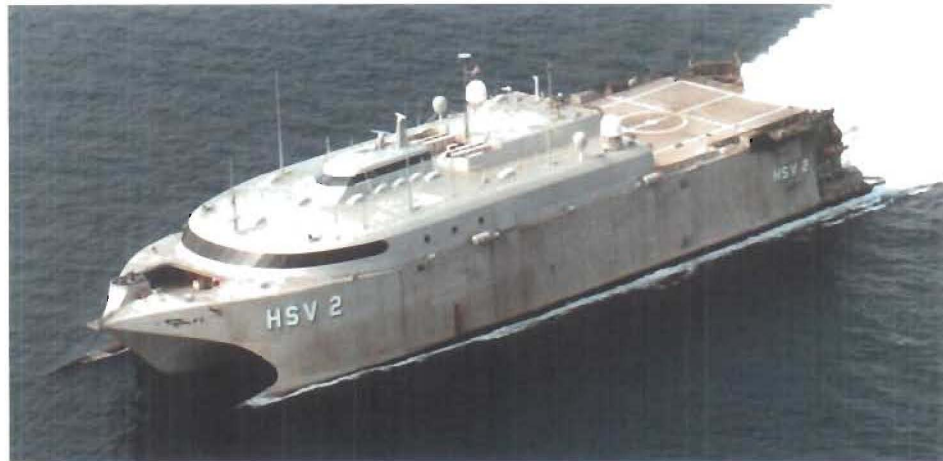
Figure 1. All aluminum high-speed vessel HSV -2 Swift
