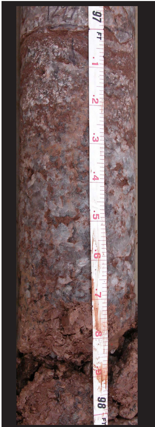
Figure 2-7. Short Desiccating-upward Cycle in H-3a. Coarse halite at 1,397.8 ft becomes finer upward. A thin reddish brown siltstone at 1,397 ft rests on an undulatory surface and is overlain by coarse halite with little clastic content.
