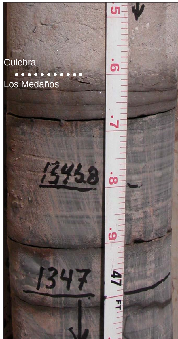
Figure 2-4 (below) Thin, Undeformed Laminae in Uppermost Los Medaños Member from SNL-6A
