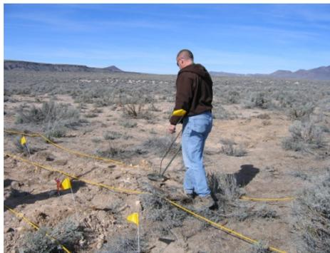
**Photo 3-2 Technician Performing Sweep with Schiebel**
