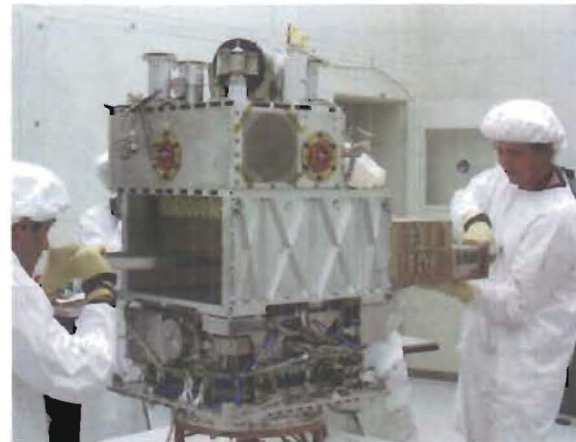
Figure 6: Integration of the LANL payload and the SSTL satellite bus, June 15 th , 2006.
