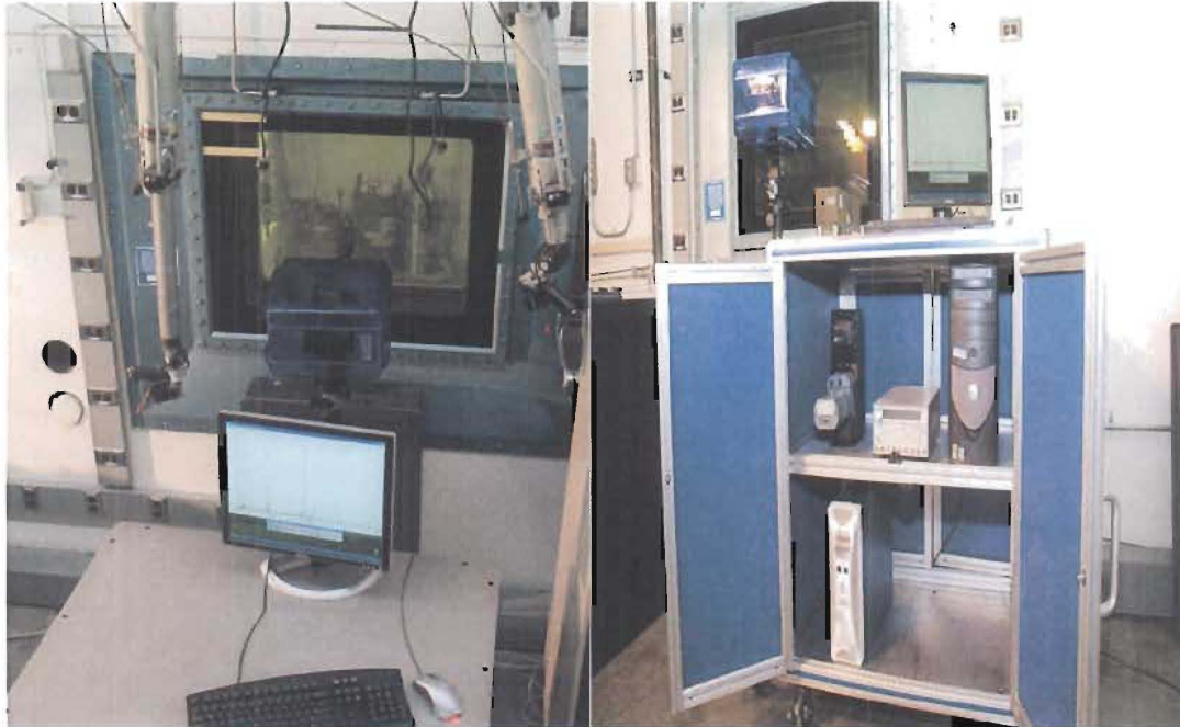
Figure 9. A prototype version of a field deployable high resolution LIBS system is shown in this picture.
