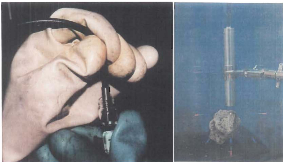
Figure 2. On the left hand side of this figure is shown the end of a LIBS fiber optic probe where the analyst is analyzing a solution containing plutonium. On the right hand side of this figure is shown another fiber optic probe directed onto the surface of a rock for analysis. The small white spot is the plasma being generated on the surface of the rock. In both cases, the probe contains the telescope optics for focusing the laser and collecting the emission from the plasma.
