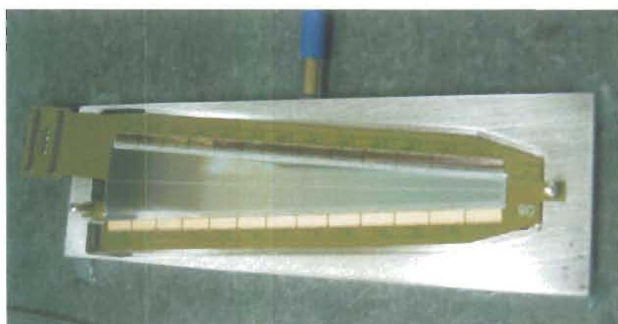
Fig. 2 FVTX wedge assembly with sensor and 13 FPHX chips.
