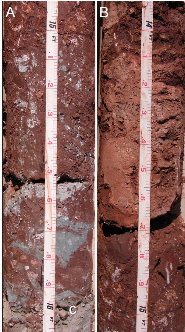
Figure 2-5. Core from M-3 at SNL-18. A - Gypsum clasts (c) at the base of M-3 at 516 ft below irregular clasts of siltstone. B - Claystone-mudstone contact at 514.7 ft.
