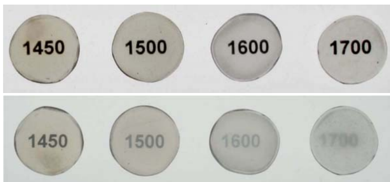
Figure 11. Transparency of specimens hot-pressed at the indicated temperatures ( ^{\circ}\text{C} ). Upper picture shows specimens in contact with text; lower, 1 cm above text.
