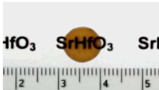
Figure 18. Contact transparency of sinter-HIPed \text{SrHfO}_3\text{:Ce} disk in direct contact with back-lit text.
