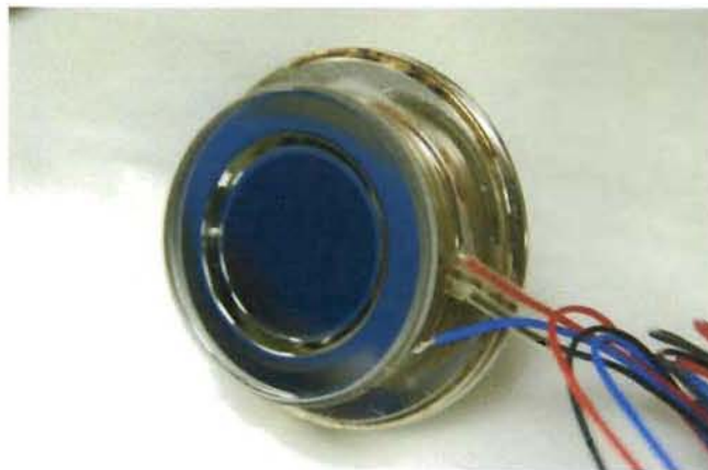
Figure 1. Near infrared wavelength enhanced S-25 photocathode cross delay line sensor.
