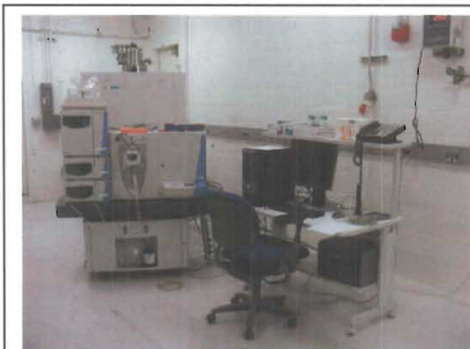
Figure 3) A ThermoFinnigan LC/ESI/FT Mass spectrometer. The ppm mass accuracy allows metabolites to be identified by their masses or their calculated formula weights, thus greatly aiding in the identification of previously unknown metabolites.
