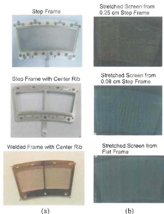
Figure 7. (a) Foil holder design evolution including stepped frame, ribbed-stepped frame, and welded ribbed frame design and (b) stress contours in flattened screens that have been previously stretched in various foil holder assemblies.
