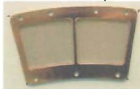
Figure 15. Photographs of a welded frame foil holder before and after the phase 3 acoustic test.
