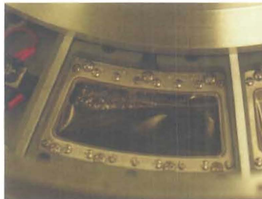
Figure 14. Broken foils encountered during the phase 1 acoustic tests.
