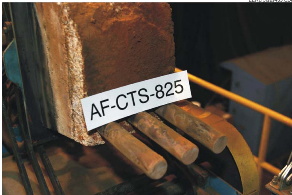
Figure 4. Probe bank at end of Test 5, 1050°C.
