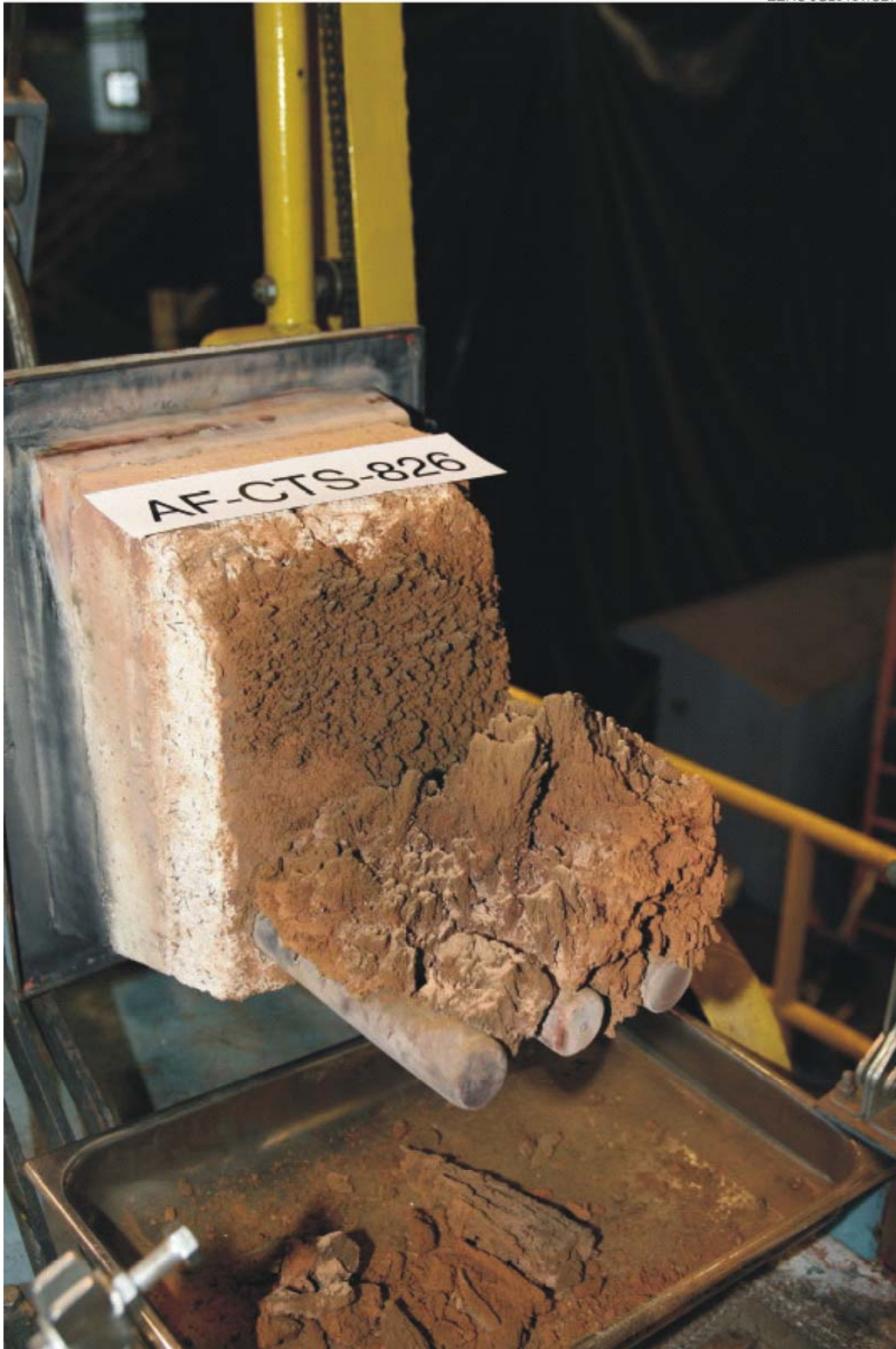
Figure 5. Probe bank deposit formed in Test 6, at 1120°C.
