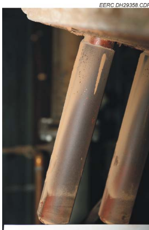
Figure 22. Front side of the ash-fouling probes removed from EERC CFBC convective pass.
