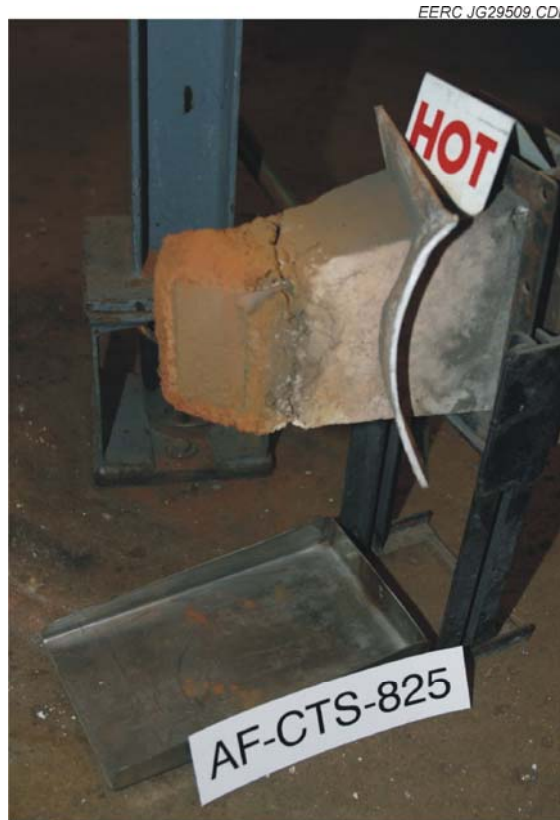
Figure 6. Slag probe utilized in Tests 5 and 6.
