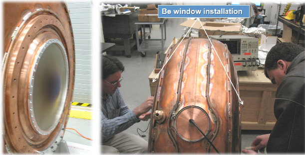
Figure 6: Beryllium window installation and (left) installed window on MICE cavity.
