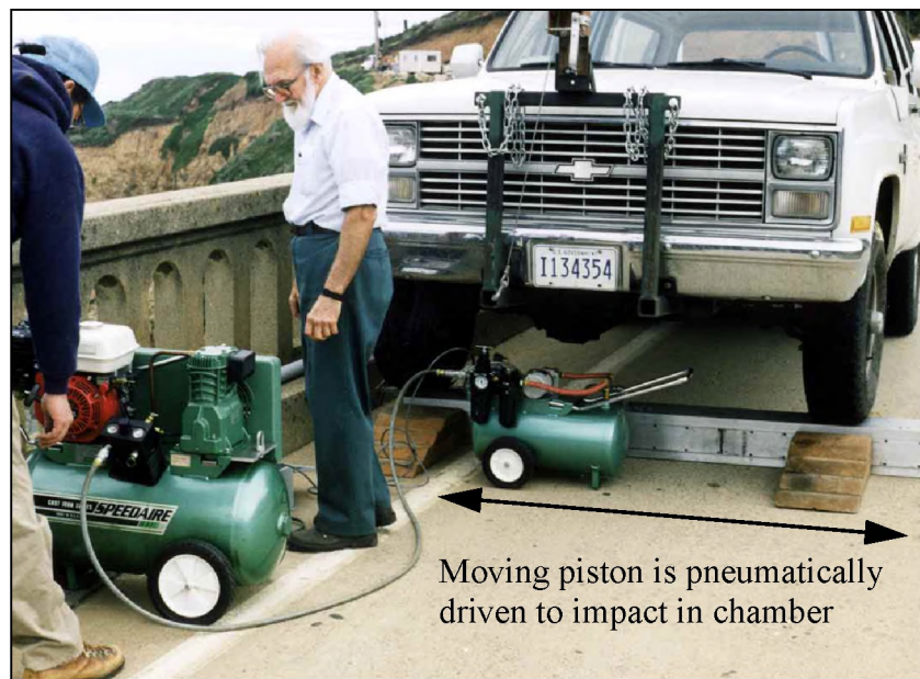
FIGURE 61. USGS pneumatic impact hammer for transverse bridge excitation.
