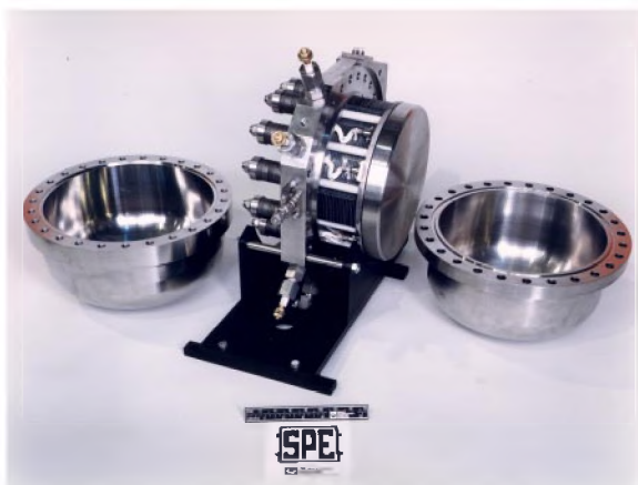
Figure 9. Integrated Propulsion Test Article (IPTA). Built as a demonstrator for a propulsion electrolyzer. Anode feed, 3000 psi balanced pressure. Used the old style hardware and therefore required the dome and the nitrogen system (not shown). It was in all respects a scaled down version of the oxygen generator for the submarine.
