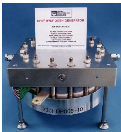
Figure 11. High pressure, anode feed hardware. Metal laminate assembly capable of 3000 ASF current density. Developed for life support, the technology is conducive to extremely lightweight developments. The assembly was designed for anode feed operation with the hydrogen being produced at high pressure and the oxygen at ambient. The water make-up does not require a high pressure pump. The same technology is used for the 200 W passive water feed electrolyzer for LLNL. Portable lightweight electrolyzers are taken one step further towards new applications.
