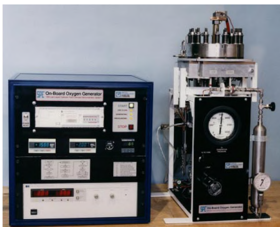
Figure 7. OBOGS demonstration system package. The system could fill a 250 ml tank to 1800 psi or vent directly to ambient through a back pressure regulator. It was capable of automatic start and stop based on a pre-determined number of conditions. Sized for 200 ASF ( 0.22 \text{ A/cm}^2 ) operation.
