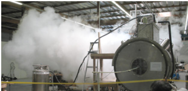
Figure 7: Quench during spectrometer solenoid training.
