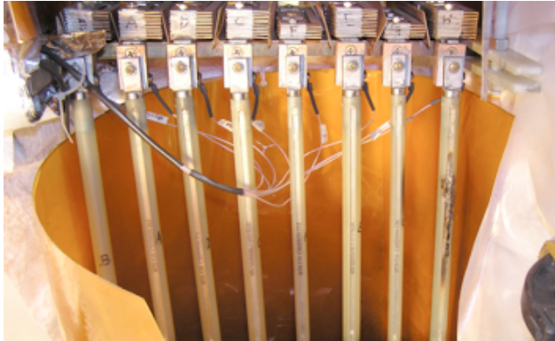
Figure 6: Burned out HTS lead (right side).
