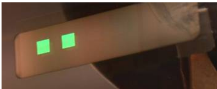
Figure 30: First OLED device with a OVJP deposited emission layer made at UDC
