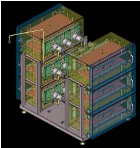
Figure 21: Six source ovens in two vertical stacks, mounted on a frame.
