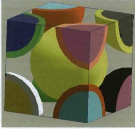
Figure 5: MCNPX model of a pebble and its neighbors using Body-Centered-Cubes representation (reflective boundary condition applied).
