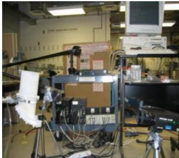
Figure 23 Pictorial View of Laser-based PIV Experimental Set Up and Instrumentation
