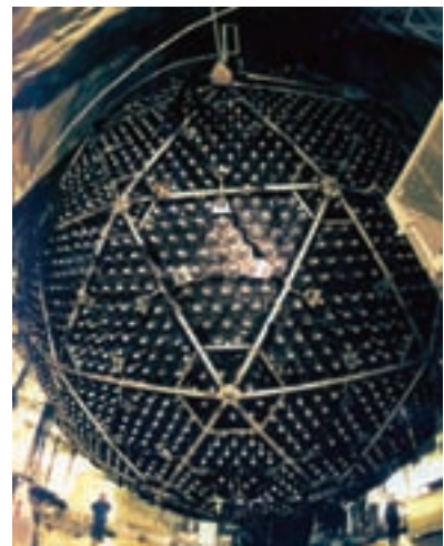
Figure 13. By filling this 12-meter sphere at SNO with an unusual type of heavy water and surrounding it with light detectors, astrophysicists were able to collect enough data to solve the mystery of the missing solar neutrinos. That data is now archived at NERSC for future re-analyses.
