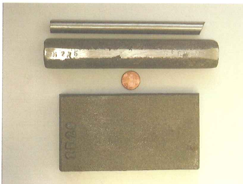
Fig. 2 – Keel bar of as-cast CF8C-Plus (heat N276), top, and cast block of HK-30Nb, bottom, with U.S. penny shown for size reference inbetween. The rod shown above the keel bar is the maximum diagonal length extracted (electro-discharge machining, or EDM) from the HK-30Nb keel bars for producing LCF specimens.
