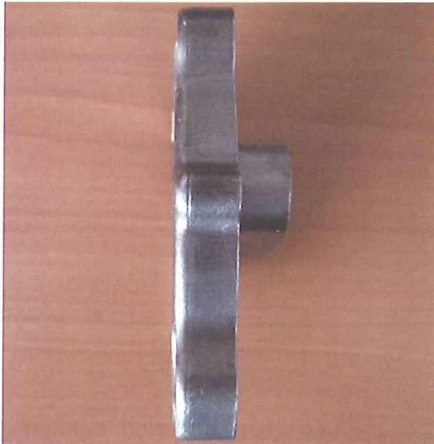
Fig. 9 – Investment cast end-cover of CF8C-Plus stainless steel for the turbocharger housing of a C-15 on-highway diesel engine, for A) outside face view, and B) side-view.
