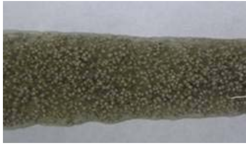
Figure 15 Uniformly distributed slurry created by the mixing system
