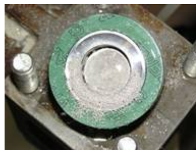
Figure 18 Proppant particles prevent the valves from fully close
