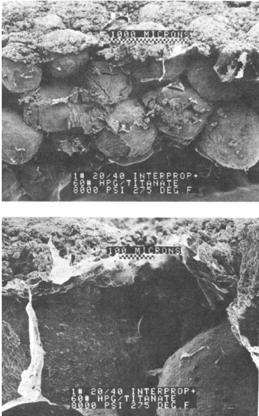
Figure 33 SEM photomicrograph of a proppant-core-fracturing fluid interface is showing filter cake, gel residue, and formation fines. Bottom photo is a closeup of the top surface [Penny, 1987].
