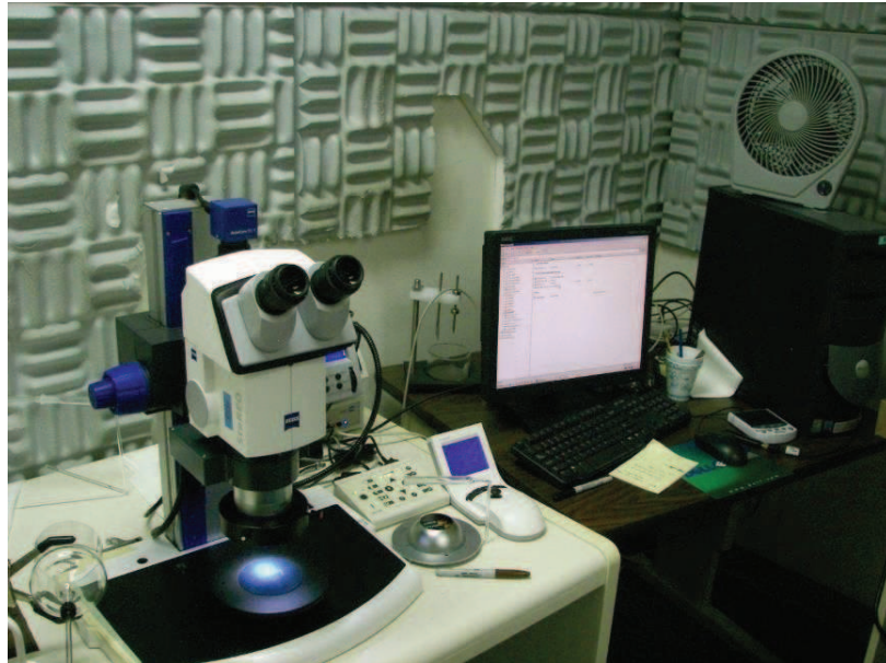
Figure 2. Zeiss Discover V12 stereoscope with Axiocam ICc1 3 megapixel digital camera setup with computer system
