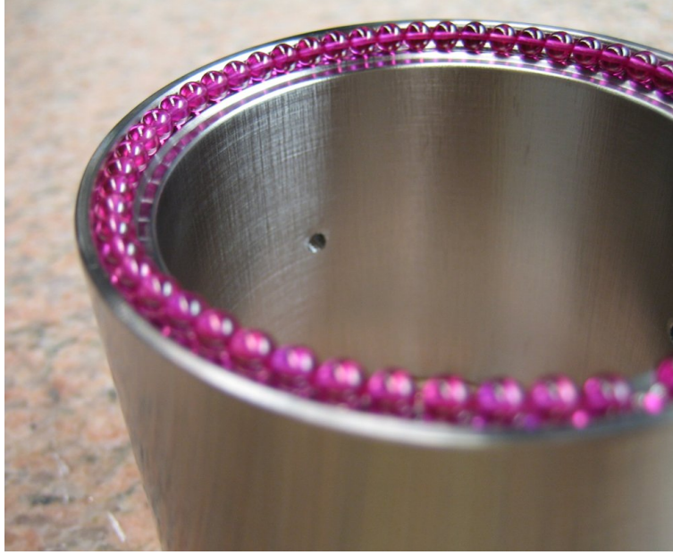
Figure 4.18. One end of a cylindrical electrode, with its bracelet of 56 ruby balls in place, contacting surfaces A' and R' , as labeled in Figure 4.15.
