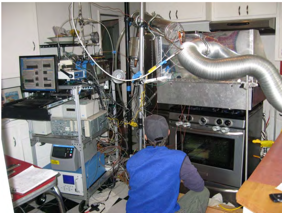
Figure 7. Collection hood installed over island cooktop
