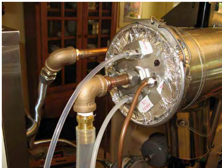
Figure 4. Outlet of dilution sampling system
