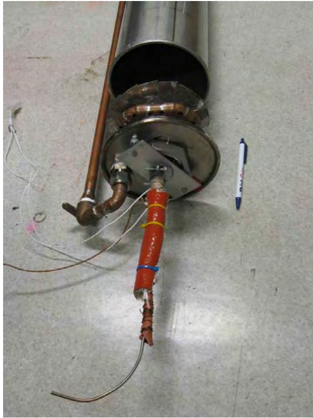
Figure 3. Dilution sampler inlet configuration
