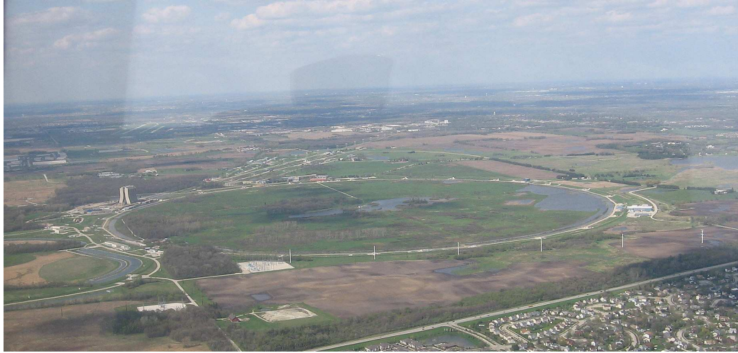
Figure 3.1: Aerial view of the Tevatron accelerator. The Tevatron ring is the large circle in the center of photograph. At the top of the circle is CDF, and to the right is DØ. At the left is part of the Main Injector. [Image courtesy of M. Prewitt]
