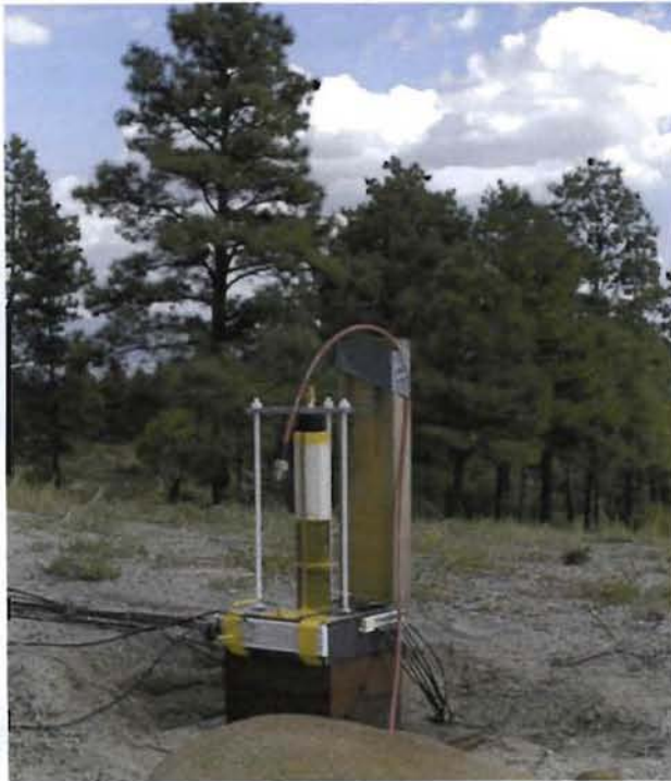
Figure 1. LANL large-scale gap test with TAGzT (yellow) fired with PBX9205 (white)
