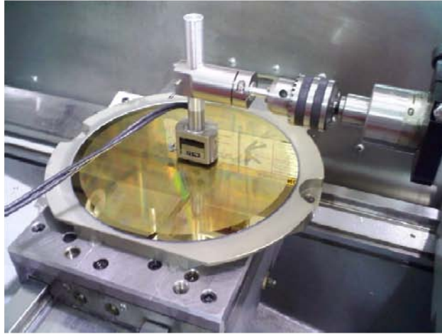
Figure 10: Experimental Setup of the Machine Grid Plate Testing.
